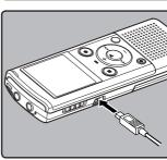
Make sure that the recorder is stopped, and then connect the USB cable to the connecting port on this recorder.
